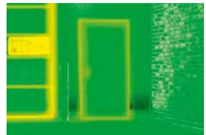
Far smaller energy loss thanks to thermally separated door
