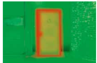
Visible energy loss without thermally separated door
