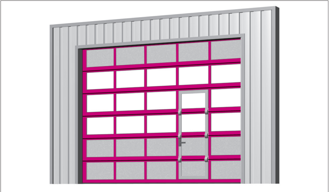
SL door with glass, sandwich board 16 mm and integrated wicket
