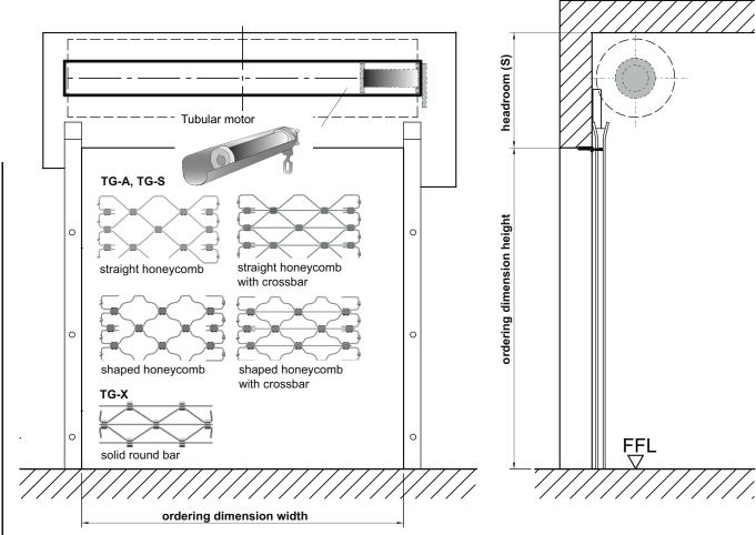
Standard installation: Mounted behind the door opening
