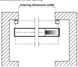
Special installation: Mounted in the door opening (substructure on site)
