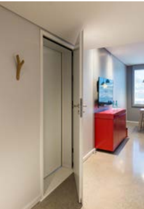
Sound insulation par excellence by means of access doors installed behind each other.
