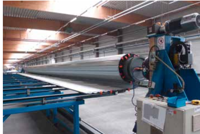
By default roller doors can be produced in 11.5 x 12 metres. Door widths up to 18 metres can be realised on request.
